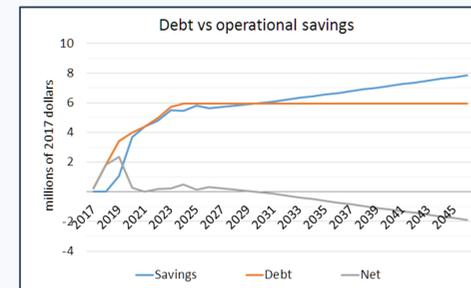
Figure 7. Sensitivity analysis for conversion to hot water system with heat recovery chillers
