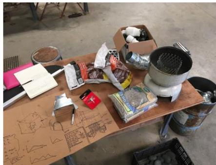
This is the design for our first prototype using a propane tank that is cut in half. This design was without air intake ports for baseline testing and then modified to open airflow at the base of the burner for further testing.
