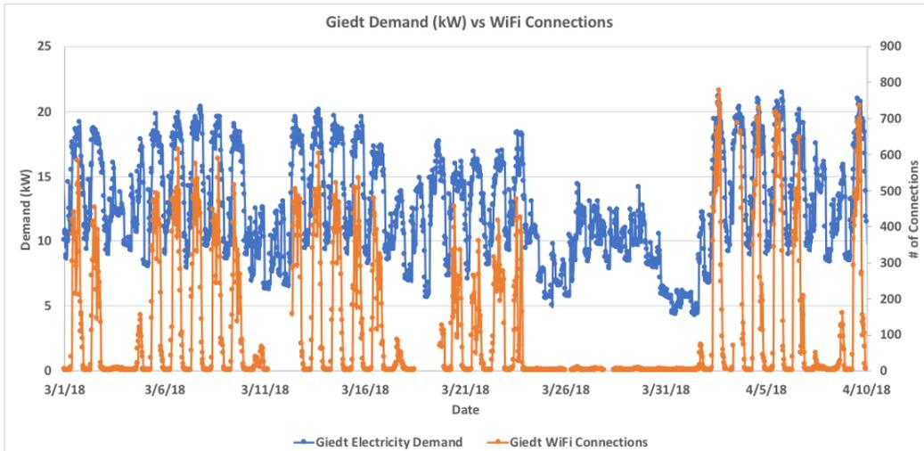
Figure 10: WiFi connections vs building electrical demand for Giedt Hall
