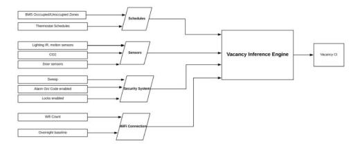
Figure 8: Flow Diagram of inputs and outputs of Vacancy Inference Engine (VIE)
