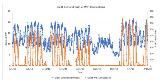
Figure 10: WiFi connections vs building electrical demand for Giedt Hall
