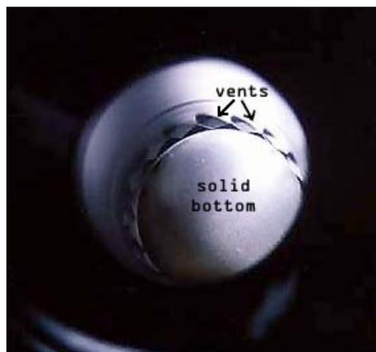
**Figure 1:** Interior design for popcorn roaster. For effective roasting, the vents are recommended to be placed on the sides.
