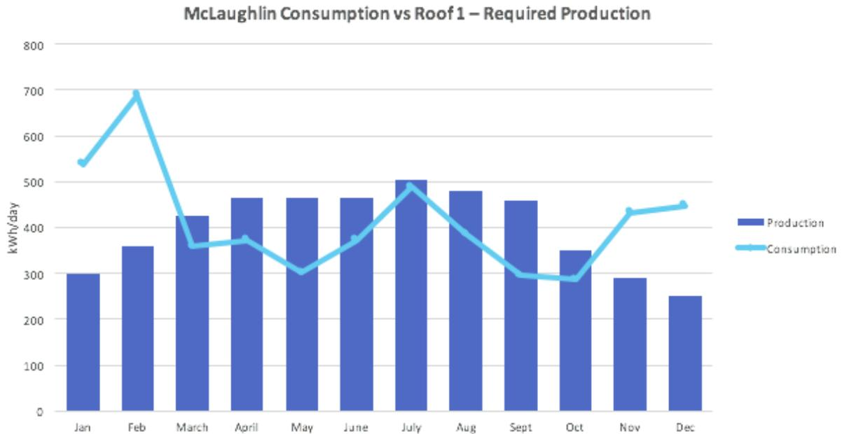
Figure 4. Total energy consumed by the reserve annually compared to the modeled production of the Roof 1 PV system to meet demand.
