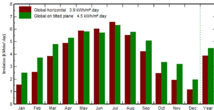
Figure 3: Graph showing increase in irradiance for 30° south tilt of panels
