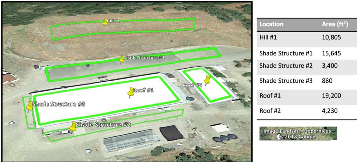
Figure 2: Potential Photovoltaic Infrastructure Locations
