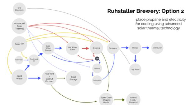
In order to help our client visualize the process, we made conceptual designs incorporating the technologies we discussed throughout the quarter. The first graphic represents a system where waste heat recovery, water reuse, and conventional solar hot water are used to minimize fossil fuel use. In the second option, advanced solar thermal replaces propane and minimizes grid reliance for cooling.
