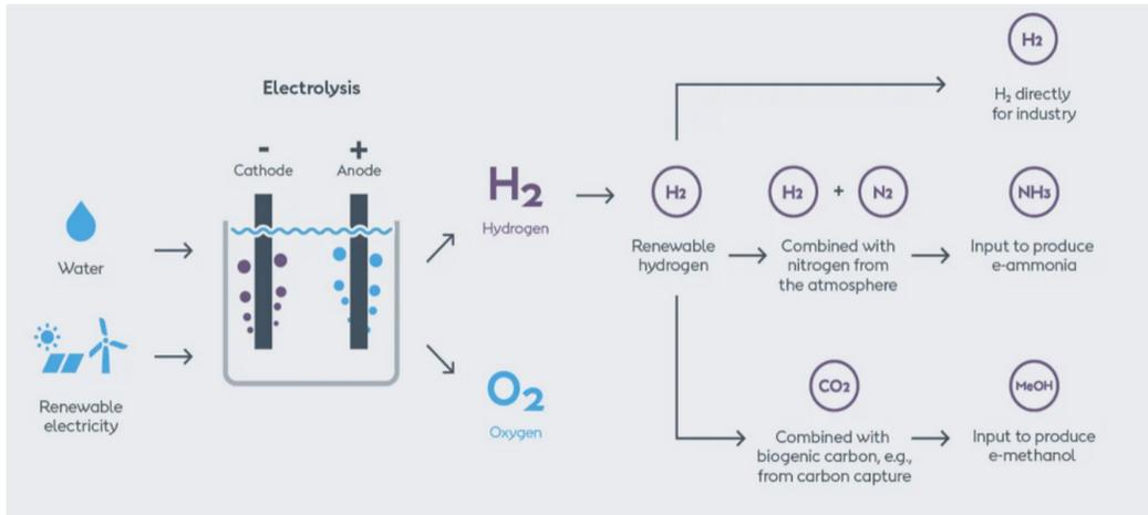
P-t-X refers to converting renewable electricity into carbon neutral substitutes for fossil fuels. The process makes green hydrogen, which can be converted to other fuels.
