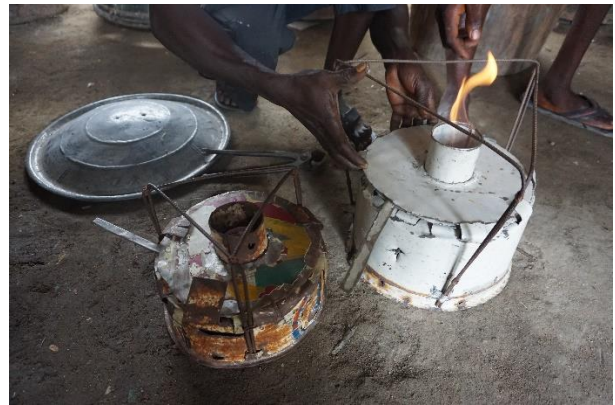
The first ethanol stove prototype, built using familiar coalpot design and fabrication techniques
