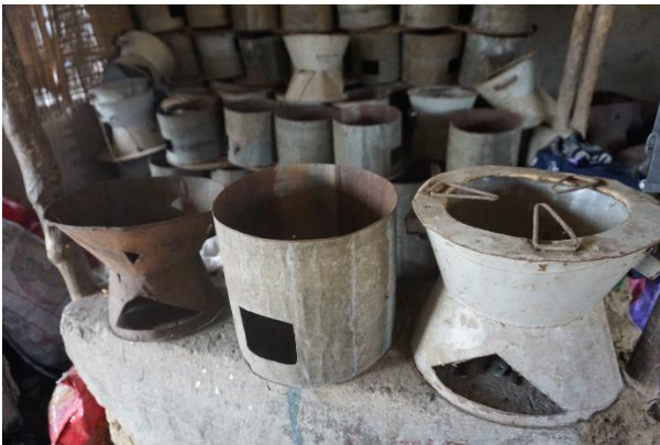
The coalpots our fabricators normally produced using sheet metal and simple bending and folding techniques
