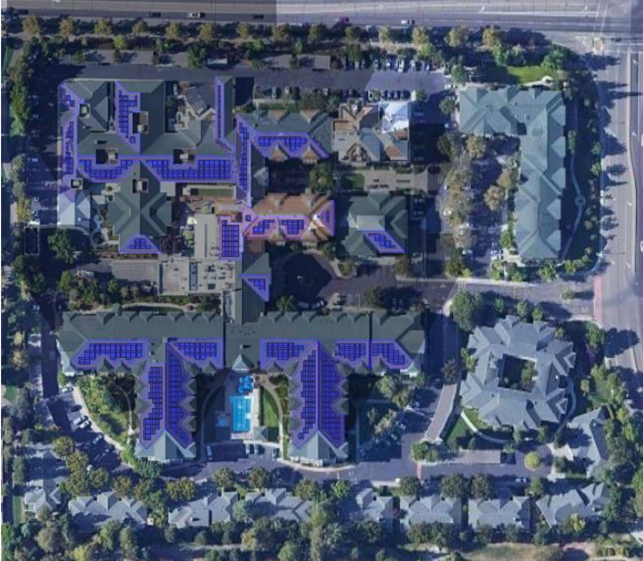
Figure 4: HelioScope model 2 – main facility rooftop considering north, south, and east-facing surfaces. Hanwha 470-watt modules used here.
