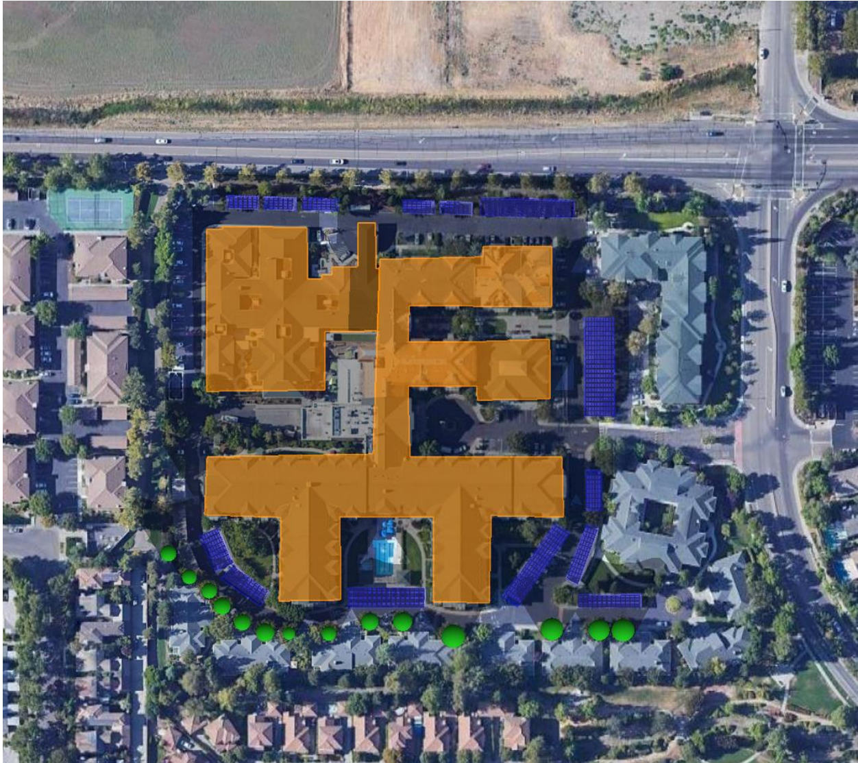
Figure 7: Maximum carport capacity, showing carports (blue), and for shade modeling, structures (orange) and trees (green).
