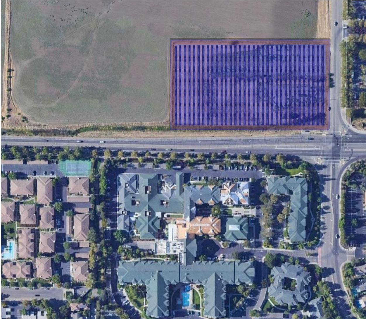
Figure 8: Model 6 showing proposed single-axis tracking (SAT) PV system north of W Covell Blvd.
